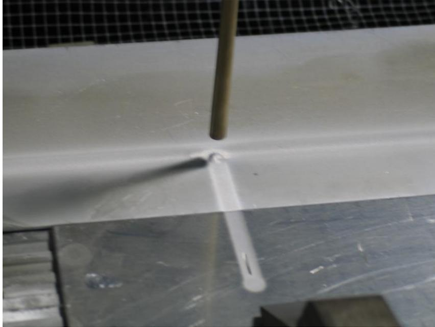
Figure 8: Cold Spray Deposition Trial with 2024 Al Powder (400 mesh)
