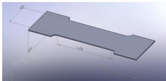
Figure 2: Solidworks Coupon Model
