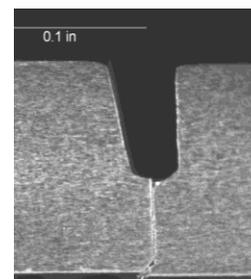
Figure 5: Fatigue Crack Macro (side)
