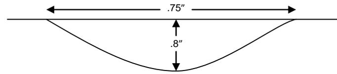
Figure 3: Pre-Crack Dimension (front)
