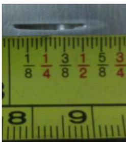
Figure 4: Fatigue Crack Width
